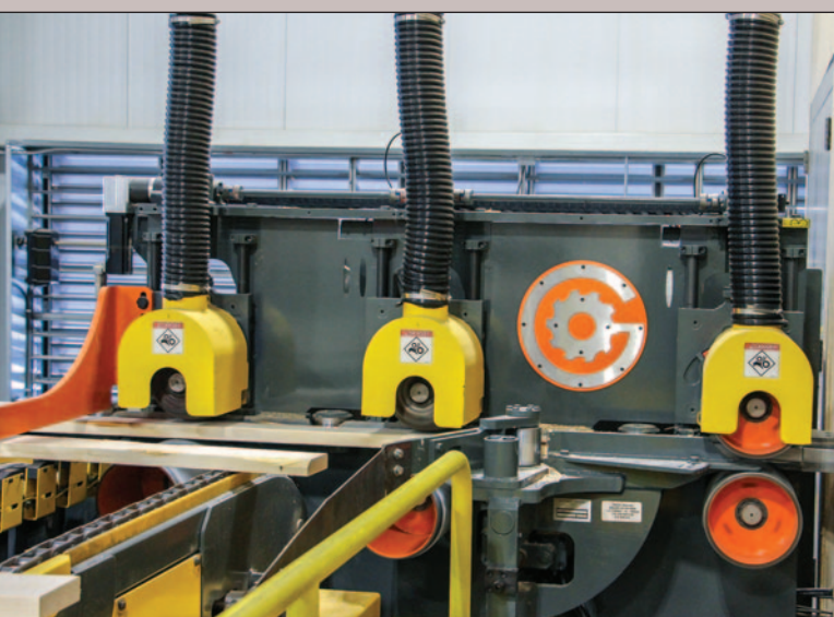
Pull through Gilbert planers plane lumber to near net sizing.
